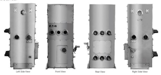
The VisoVac fault interrupter enclosure comes standard in stainless steel which is constructed for harsh vault and subsurface environments. The enclosure is also available in revolutionary molded high density polyethylene (HDPE) using patent pending technology with a safe touch exterior.
